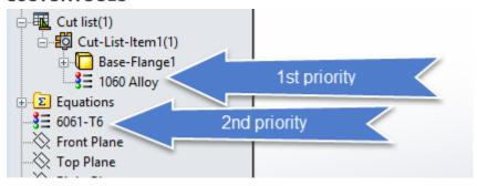
In this case 1060 Alloy would be used as value for material in the output file.
